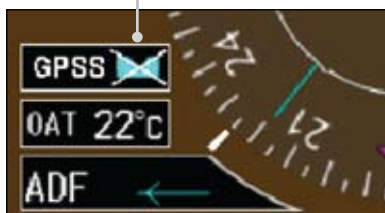
Figure 5-30 GPSS Emulation Indication
